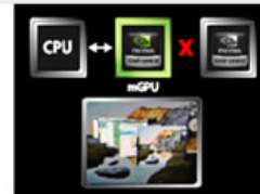
Hybrid Power switches off add-on card VGA for power saving under lower operation
