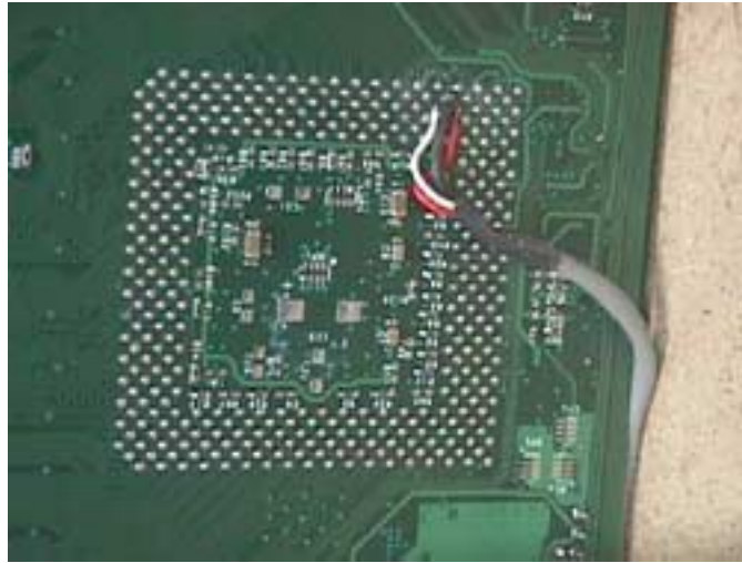
Figure 7-15. Back side of motherboard with PGA370 connections
