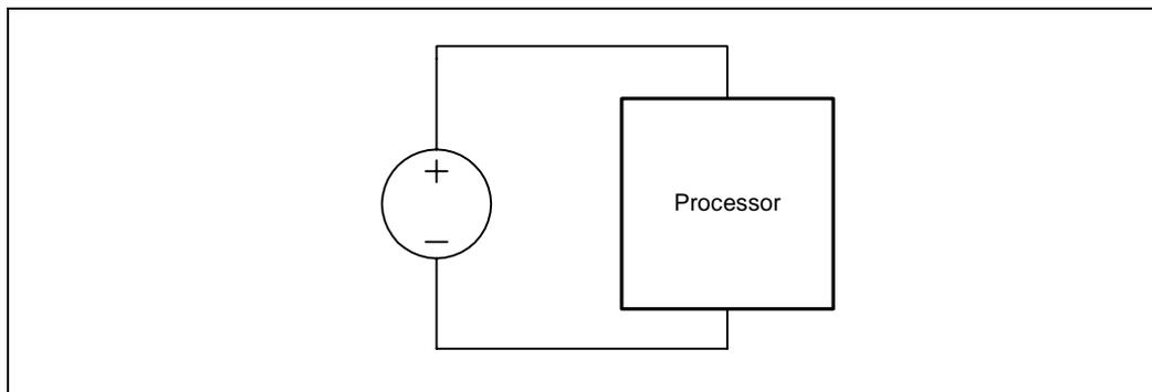
Figure 5-2 shows the recommended system baseboard solution involving local voltage regulators. Each voltage regulator solution can be either a voltage regulator module (VRM) or an embedded voltage regulator (VRD) depending upon the specific requirements of the board designs. It is recommended that board designers follow the guidelines in VRM 8.5 DC-DC converter design guidelines document.
