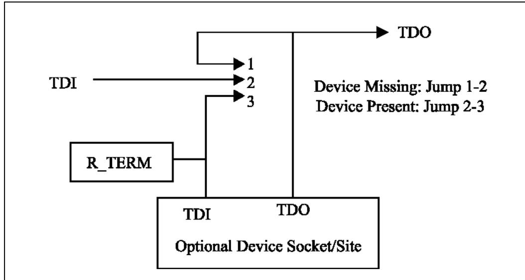
Figure 3-10. 4-Pin Jumper Bypass
