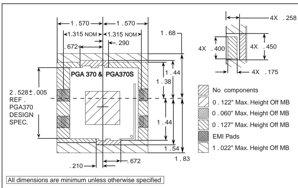
Figure 2-3. Socket 370 Volumetric Keepout
