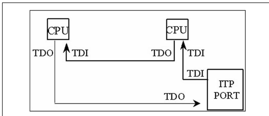
Figure 3-9. TDO 3-Pin Jumper Bypass
