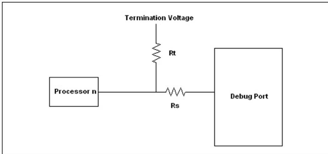
Figure 3-7. RESET# Signal Termination
