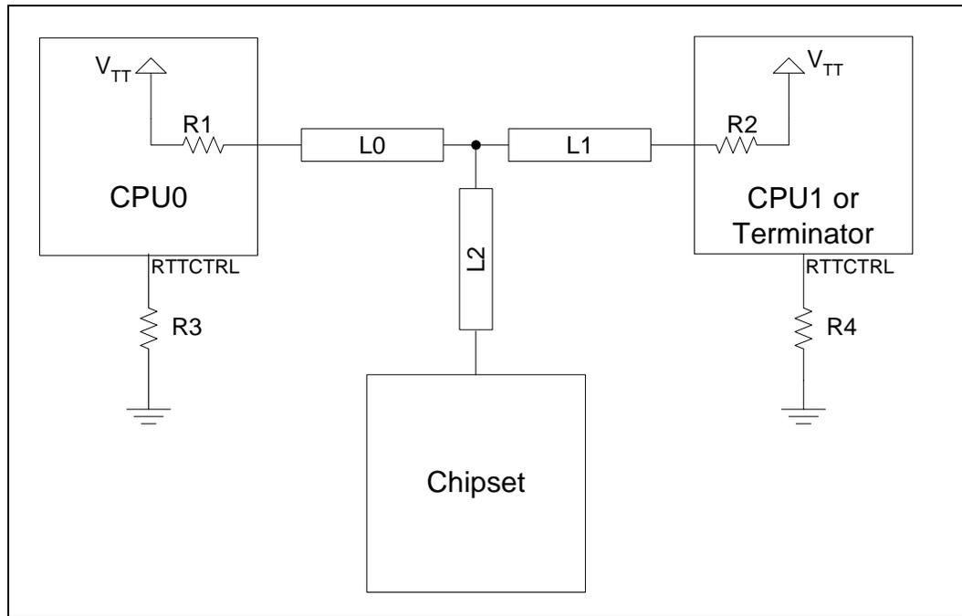
Table 3-5 contains the length specifications for the segments of the T-topology. Please note that lengths L0 and L1 must be length matched to within 0.25 inches. Table 3-6 contains the component values which should be used for this topology.
