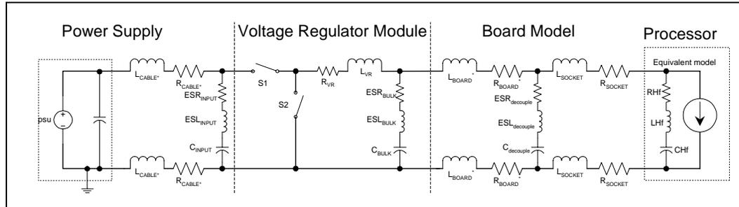
Both VRD and VRM solutions should be designed in conjunction with the recommended load model referenced in Figure 5-4.
