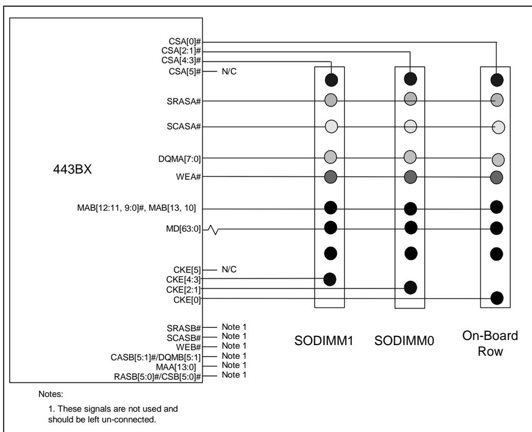
Figure 6. SDRAM - Two SODIMMs
