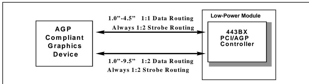
Figure 15. Signal Layout Recommendations
