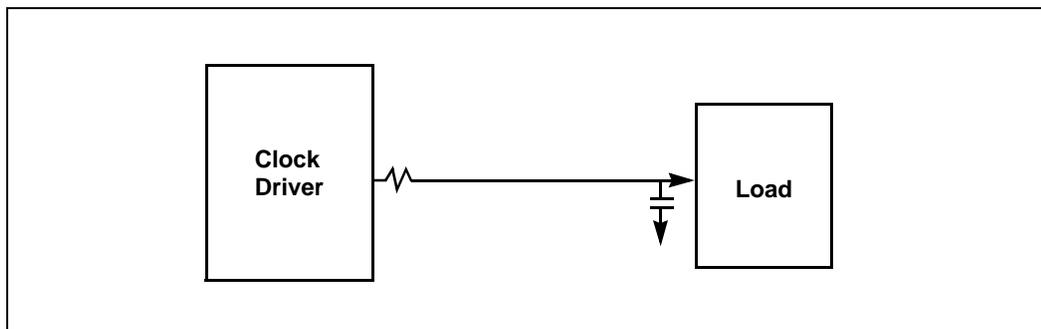
This optional layout implementation is suggested to accommodate clock tuning, HCLK & PCICLK from CK100-M and SCLK from CKBF-M. This will allow the designer to tune the individual clock signals to minimize EMI and allow for variations in impedance, skew and loading.
