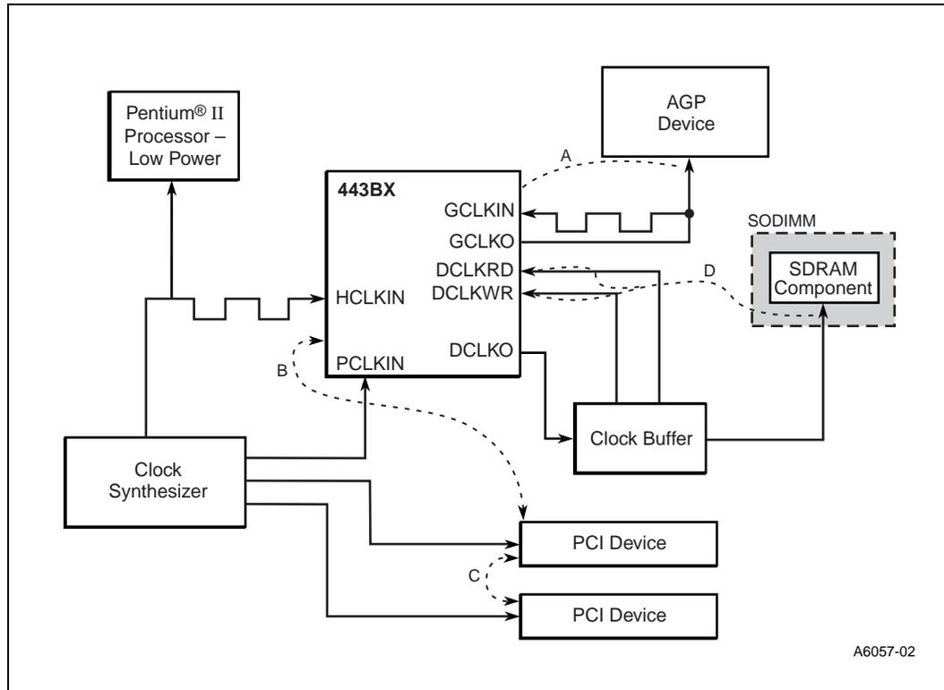
Figure 11 shows a simplified clocking layout for the timing specifications. The recommended trace lengths are given in the Note on page 30. See Table 9 for the clock skews.
