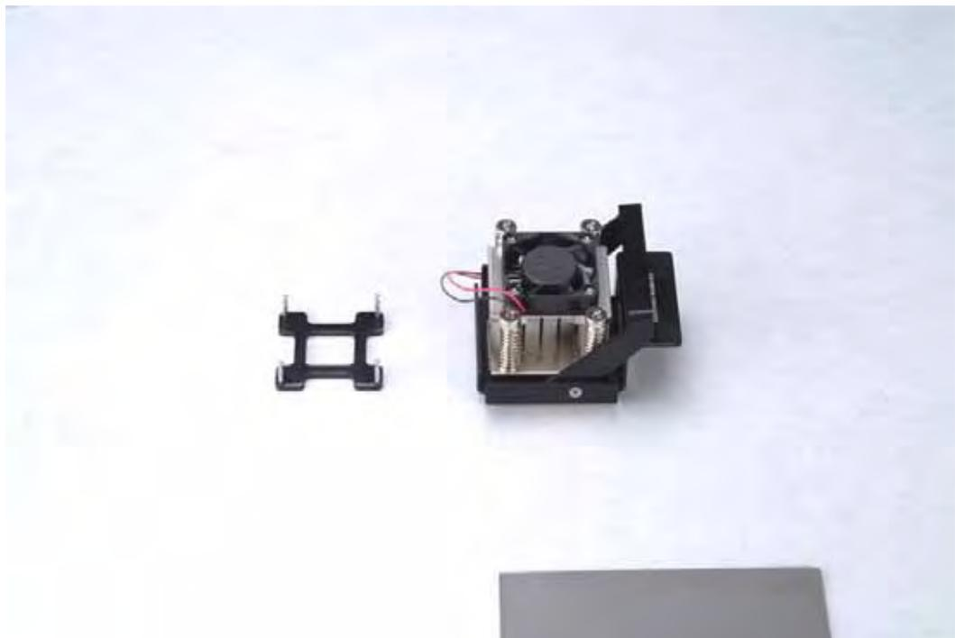
2. Examine the base of the heatsink, where contact with the processor die is made. This surface should be clean of all materials and greases. Wipe the bottom surface clean with isopropyl alcohol.
