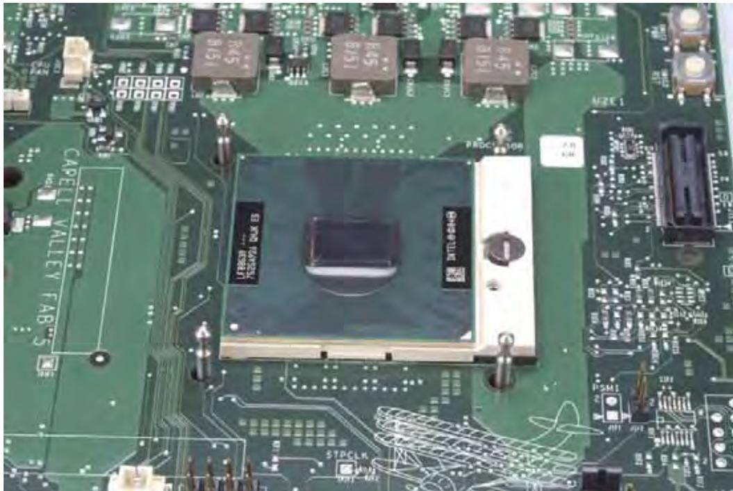
4. Clean the die of the processor with isopropyl alcohol before the heatsink is attached to the processor. This ensures that the surface of the die is clean.
