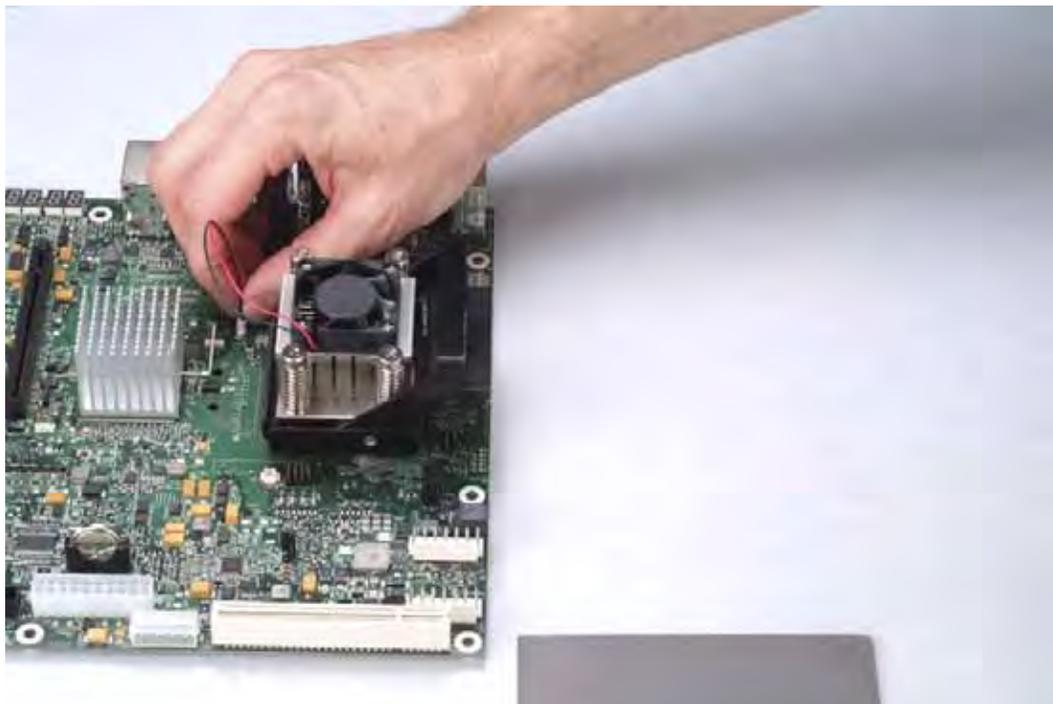
Figure 12. Completed Assembly
