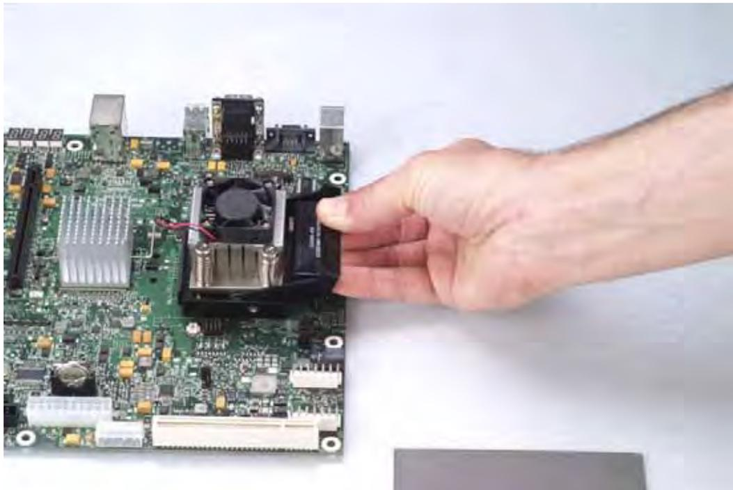
8. Plug the fan connector for the heatsink onto the CPU fan header (J3C1) on the motherboard.
