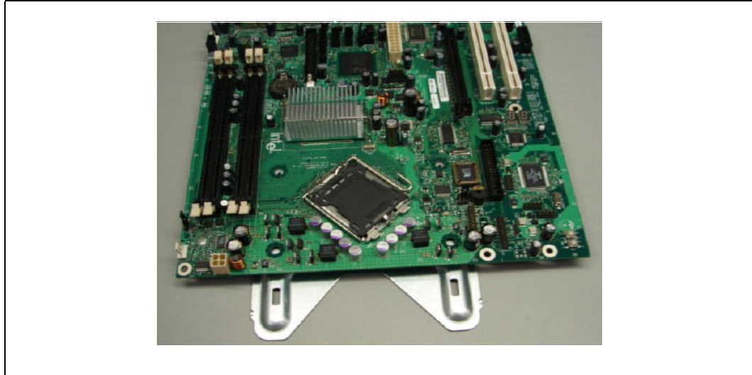
Figure 20. BTX board alignment on SRM
