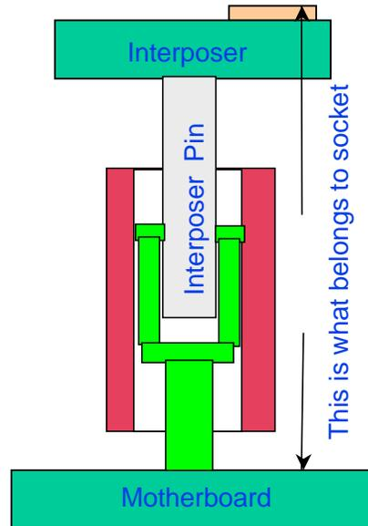
**Figure 9: Socket mated self-inductance**
