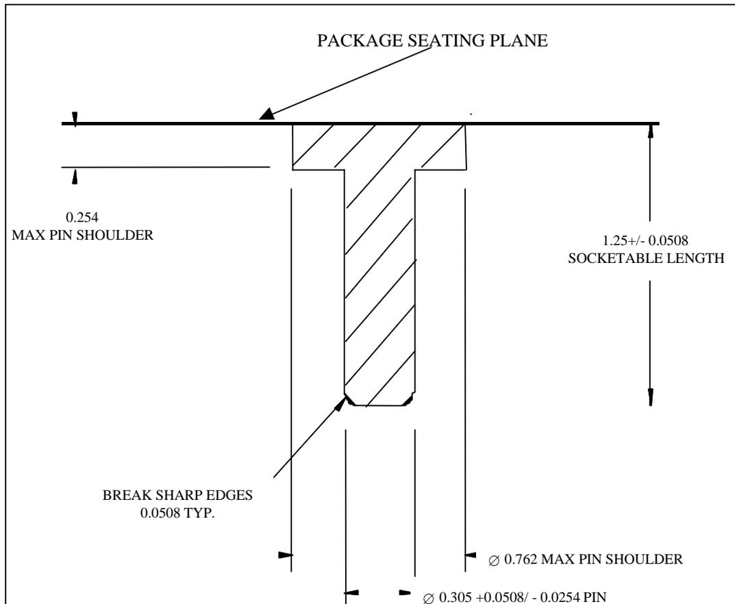
**Figure 3: Pin shoulder drawing for 615-pin Micro-PGA and 495-pin Micro-PGA packages.**
