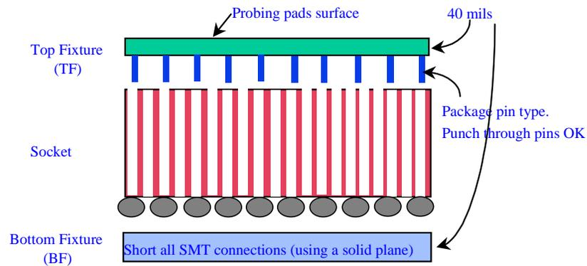
**Figure 10: Cross-sectional view of the top and bottom L fixtures**
