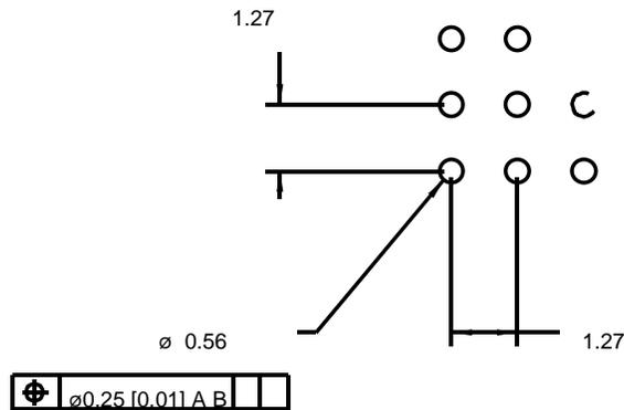
Detail A: Contact Pitch (NOTE: TP call out is for array position w.r.t. datums A and B)
