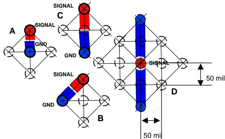
**Figure 11: Top L Fixture probing pad design (50 mil grid pattern)**
