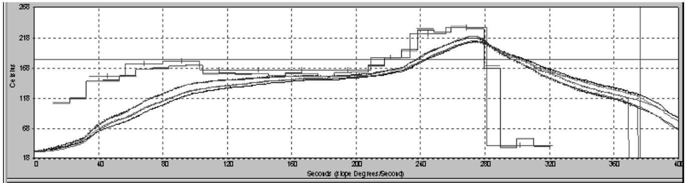
**Figure 8: Typical Reflow Profile for 63Sn/37Pb solder**
