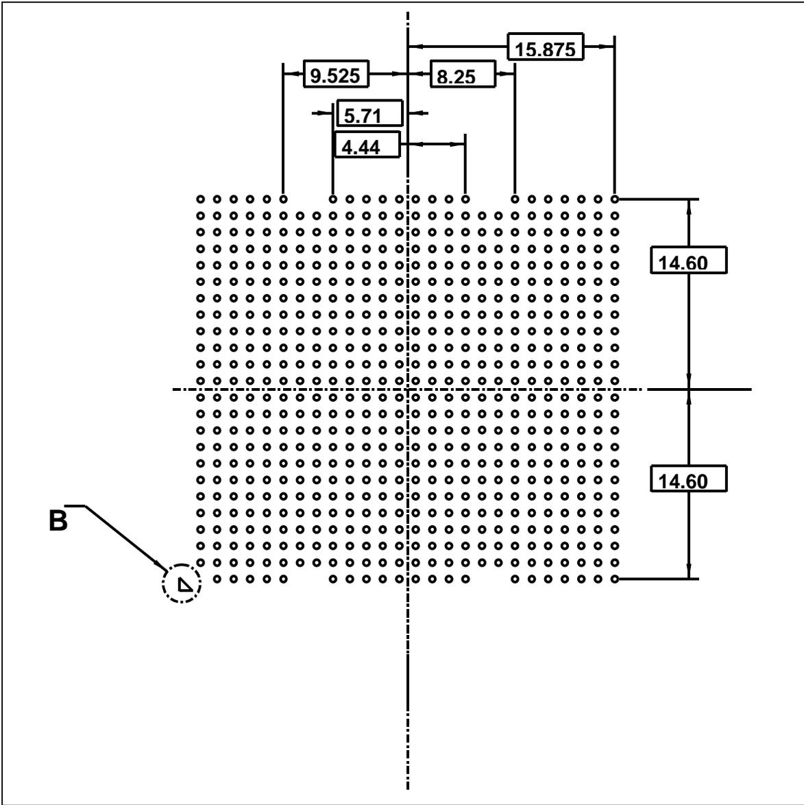
Figure 4: 615-pin Micro-PGA contact array
