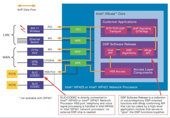
Example Application and VoIP Data Flow using the Intel® IXP421 or IXP425 network processor and the Intel® IXP4XX DSP Software Release
