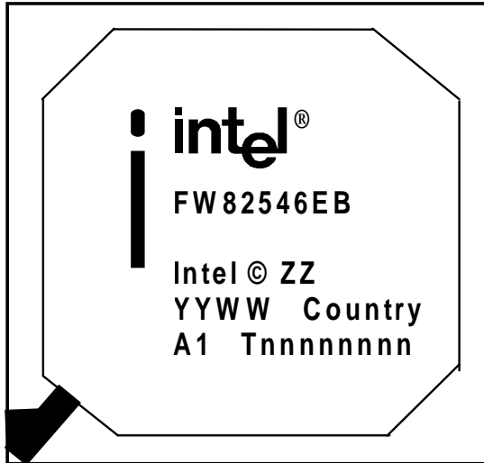
Figure 14. 82546EB Device Identification Markings
