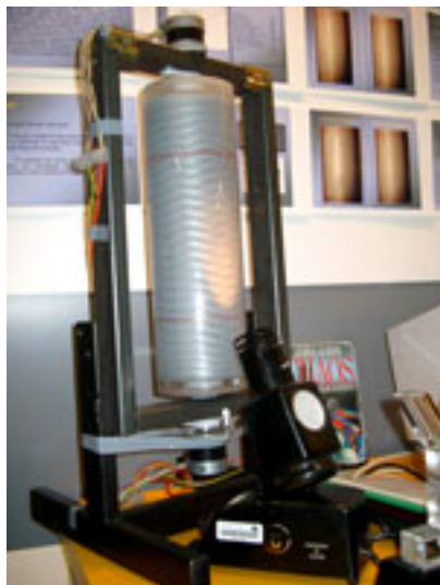
The apparatus has two independently rotating cylinders.
