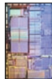
Intel486 ® Processor Introduced: 1989 Initial clock speed: 25 MHz Number of transistors: 1.2 million Circuit line width: 1 micron
