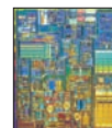
Pentium ® -4 Processor Introduced: 2000 Initial clock speed: 1.5 GHz Number of transistors: 42 million Circuit line width: 0.18 micron
