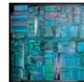
Pentium ® -Pro Processor Introduced: 1995 Initial clock speed: 200 MHz Number of transistors: 5.5 million Circuit line width: 0.35 micron
