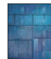
Intel ® Xeon ® Processor Introduced: 2001 Initial clock speed: 1.7 GHz Number of transistors: 42 million Circuit line width: 0.18 micron
