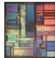
Pentium ® Processor Introduced: 1993 Initial clock speed: 66 MHz Number of transistors: 3.1 million Circuit line width: 0.8 micron
