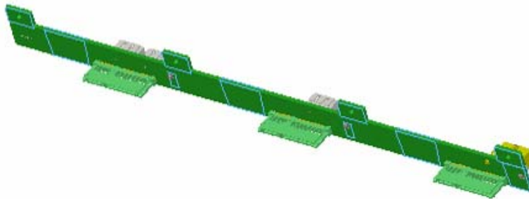
Figure 21. Hot Swap Passive Backplane - SR1530HCL/SR1530HCLR (SATA) and SR1530HCLS/SR1530HCLSR (SAS)
