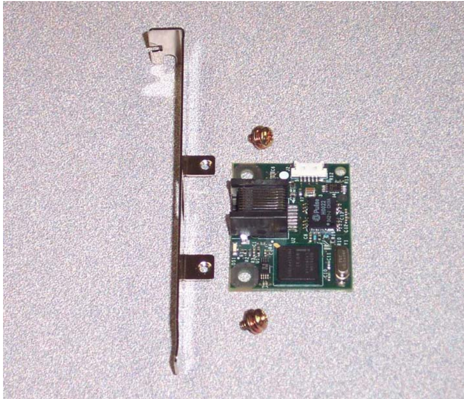
Figure 7. Intel Management Module Network Interface Card, Rear Filler Panel, and Screws
