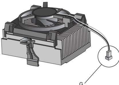
Snap the fan on the heatsink. Fan orientation is not important. Connect the processor fan cable header (G) to the motherboard connector.
