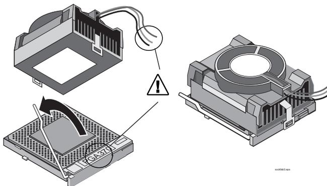
The processor fan heatsink must align properly with the 370-pin socket. Make sure to align the fan heatsink with the socket base as shown above. This will align the fan cable with the PGA370 mark on the socket. **Note: The Intel® Celeron™ processor at 533 MHz and greater ships with a 3 wire fan.**
