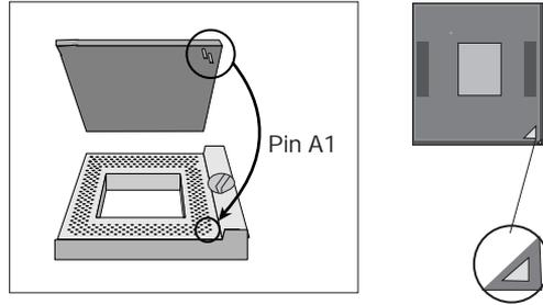
Using Figure B, place the processor into the socket. Align the processor's pin A1 with the arrow on the micro-FCPGA socket. If the processor does not drop completely into the socket, turn the actuator until the processor drops completely in.
