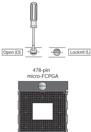
To install the processor, use a screwdriver to disengage (open) the socket actuator.
