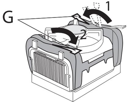
Align the heatsink and clip assembly with the retention mechanism and place it on the processor. The heatsink is symmetrical. With the clip levers in the up position (E), push down on all four clip frame corners to secure to the retention mechanism hooks (F). Close the clip levers (G) (levers require force to be completely closed).
