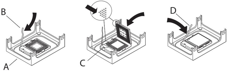
Install the processor retention mechanism (A) following the motherboard manufacturer's installation instructions. Open the socket handle (B). Install the processor by carefully aligning the pins to the socket (C). Close the socket handle (D).
