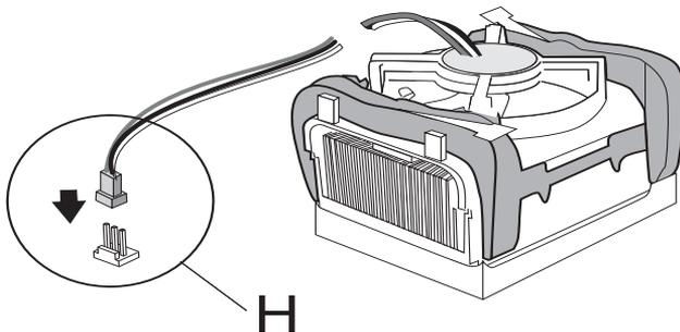
Connect the processor fan cable connector (H) to the motherboard header.
