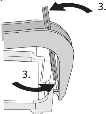
3. Push down on the clip hook and simultaneously rotate the screwdriver towards the fan heatsink to free the clip hook from the retention mechanism (RM). Repeat this process for the remaining clip hooks. Then, remove the fan heatsink.
