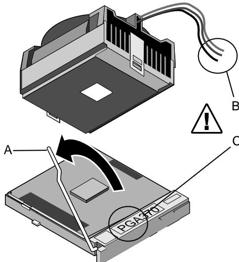
With the processor in the socket, close the handle (A). Place the fan heatsink on top of the processor. Be careful not to damage the thermal interface material. Align the fan cable (B) with the PGA370 mark on the 370-pin socket (C).
