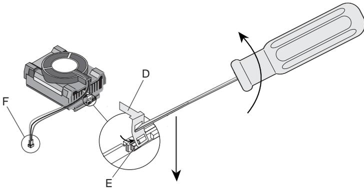
Attach the fan heatsink clip (D) to the processor socket (E). Connect the processor fan cable header (F) to the motherboard connector.
