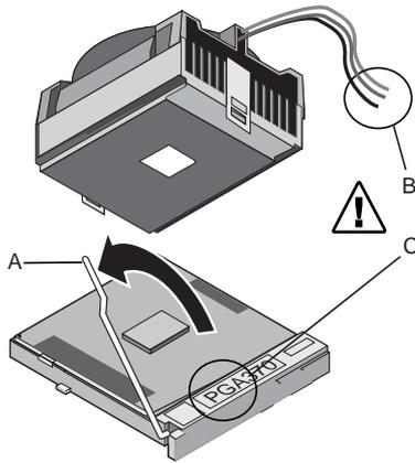
With the processor in the socket, close the handle (A). Place the fan heatsink on top of the processor. Be careful not to damage the thermal interface material. Align the fan cable (B) with the PGA370 mark on the processor socket (C).
