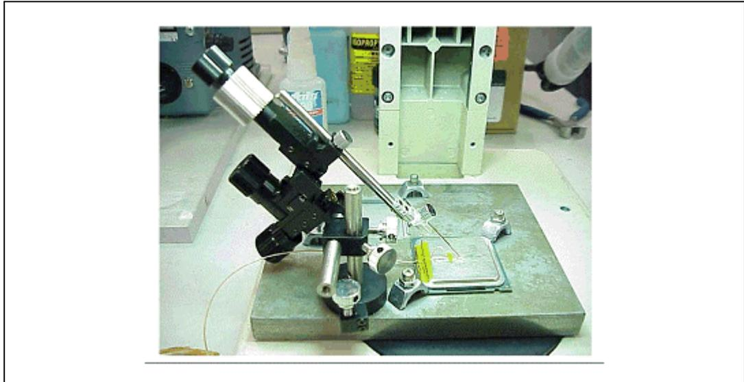
**Figure B-9. Measuring Resistance between Thermocouple and IHS**
