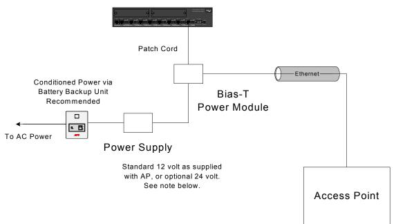
Power Over Ethernet is provided by the Bias-T module. Power for the Access Point is carried over the unused wires in a standard 4 pair CAT-5 cable. The Bias-T module is inserted in-line with the standard CAT-5 10baseT cable connecting to the Access Point. The power supply, rather than plugging directly into the Access Point, then plugs into the Bias-T module.
