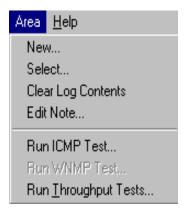
Use the menu items to create or edit a site survey area, view the settings of a survey area, clear a site survey log, add notes to the survey log, run ICMP tests and run throughput (FTP) tests.
