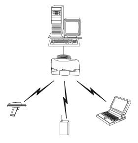
Multiple access points can coexist as separate, individual networks at the same site without interference using different Net IDs.
