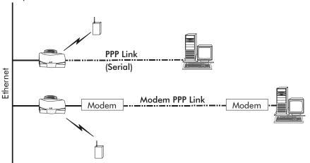
A PPP link provides the option of using a direct serial link or modem to extend wired Ethernet topologies.
