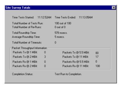
Use the Site Survey Totals dialog box to display the time the tests were started and stopped, the number of tests run, number of re-runs, total roundtrip time, average roundtrip time, total number of timeouts and the test completion status. Packet throughput information is summarized as the number of packets sent and received and the data rates for each. These values are recorded in the logfile if logging is enabled.
