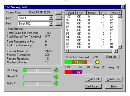
Use the Site Survey Test dialog box to specify ICMP test parameters. ICMP tests are ping tests assessing radio transmission roundtrip, delay time and transmission signal strength. Click Start Test to begin the test.
