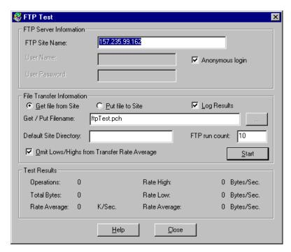
Use the FTP Test dialog box to specify throughput test parameters. Throughput tests are File Transfer Protocol (FTP) tests.
