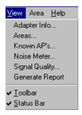
Use the menu items to view WLAN adapter driver and Firmware data, site survey areas, access points within range of a target mobile device and a graph depicting MU signal quality and to append the logfile to the report file. The status bar at the bottom of the main window can be displayed or hidden by checking or unchecking Status Bar. The tool bar buttons can be displayed or hidden by checking or unchecking Toolbar.
