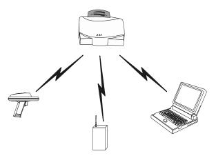
• A single access point can bridge the Ethernet and radio networks.
