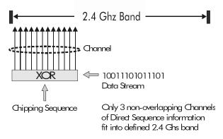
Mobile units receiving a direct-sequence transmission use the spreading code to map the chips within the chipping sequence back into bits to recreate the original data transmitted by the access point. Intercepting and decoding a direct-sequence transmission requires a predefined algorithm to associate the spreading code used by the transmitting access point to the receiving MU.
