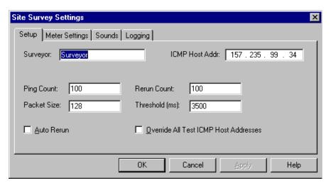
ICMP Host Addr. Enter an ICMP Host Adrress in the field provided. The default address is the default address of the AP.
