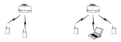
Multiple access points wired together provide a network with better coverage area and performance.
