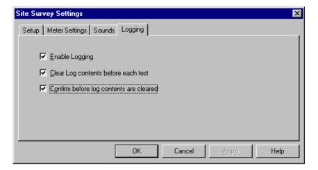
Clear Log contents before each test. Select Clear Log contents before each test to automatically clear the content of the log before a test suite is run.
