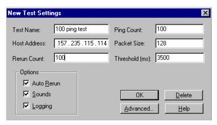
Use the New Test Settings dialog box to enter a test name, define test packet sizes, select a test ping count, enable the test Auto Rerun, Sounds and Logging features, change host address information and display the Settings property pages.
