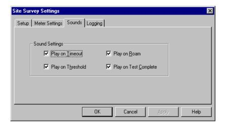
Play on Threshold. Select Play on Threshold to emit an audible threshold tone every time the threshold time is met or exceeded.
