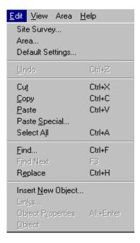
Use these menu items to edit an open Intel<sup>®</sup> PRO/Wireless 2011 LAN site survey, display a list of coverage areas within the workspace and use the Setup, Meter Settings, Sounds and Logging property pages to configure surveyor, system sounds and test data logging information. Use the menu items below Default Settings to edit the report file.
