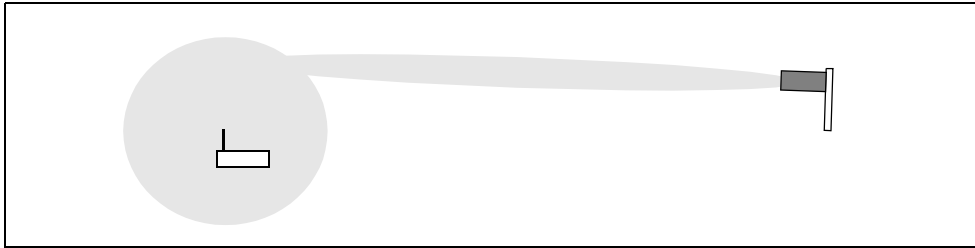
Figure 6-17: Overlapping of Coverage with Omni-Directional Antenna
