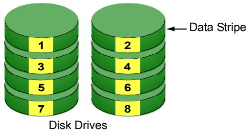
Figure 1. RAID 0 writes data to both drives at the same time
