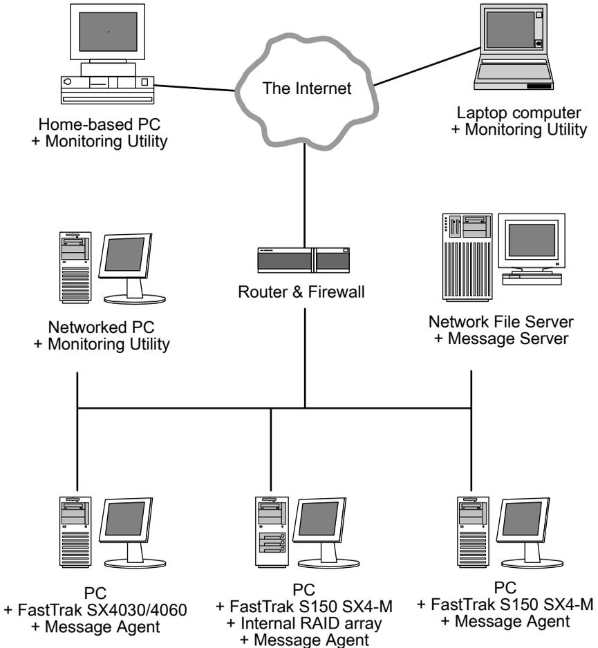
**Figure 1. Networked RAID has many installation options.**
