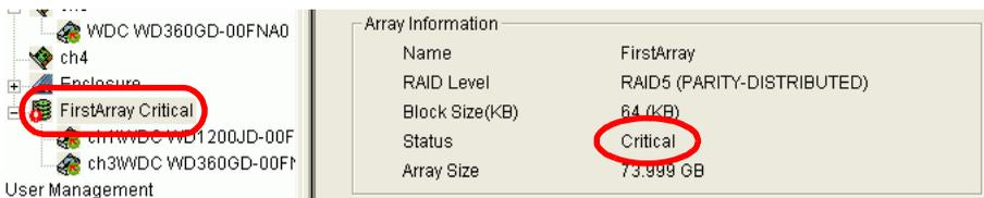
The screenshot shows a RAID management interface. On the left, a tree view displays the hierarchy: WDC WD360GD-00FNA0, ch4, Enclosure, FirstArray Critical (circled in red), ch1WDC WD1200JD-00F, and ch3WDC WD360GD-00F. On the right, the 'Array Information' window shows the following details:
