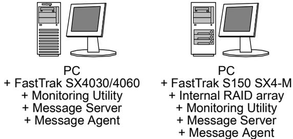
**Figure 3. PCs with Internal RAID.**
