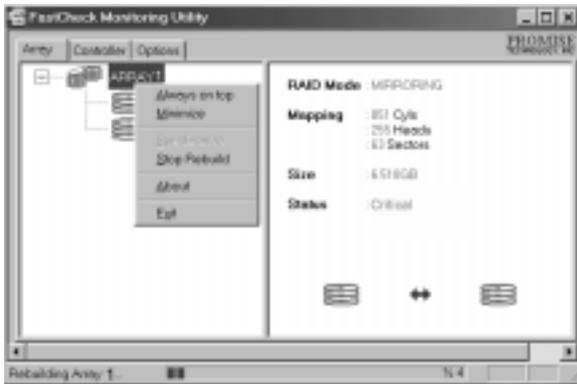
**NOTE:** When a “spare” unassigned drive is present on the FastTrak66, a rebuild will automatically be performed from the remaining working drive.
