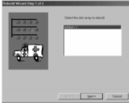
If there are multiple arrays defined, you must select the proper Array #. Press Next button to proceed to Step 2 of Rebuild Wizard or Cancel button to stop.
