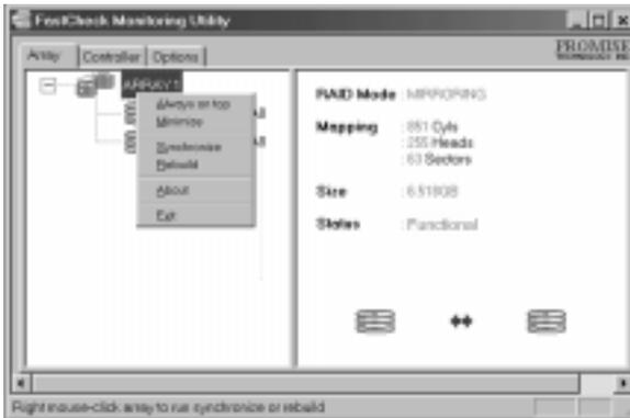
From this menu, users may choose to have the Window appear on top, Minimize, Synchronize mirrored drives, Rebuild a mirrored array, About check version #, or Exit.
