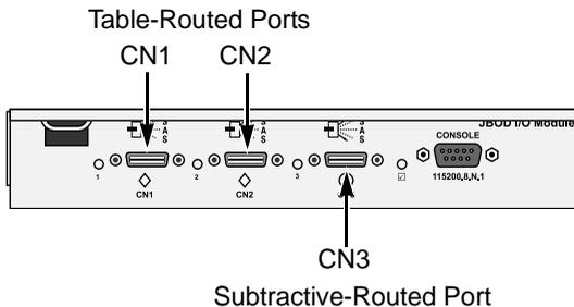
**Figure 10. VTrak J300s I/O modules have two table-routed ports and one subtractive-routed port**
