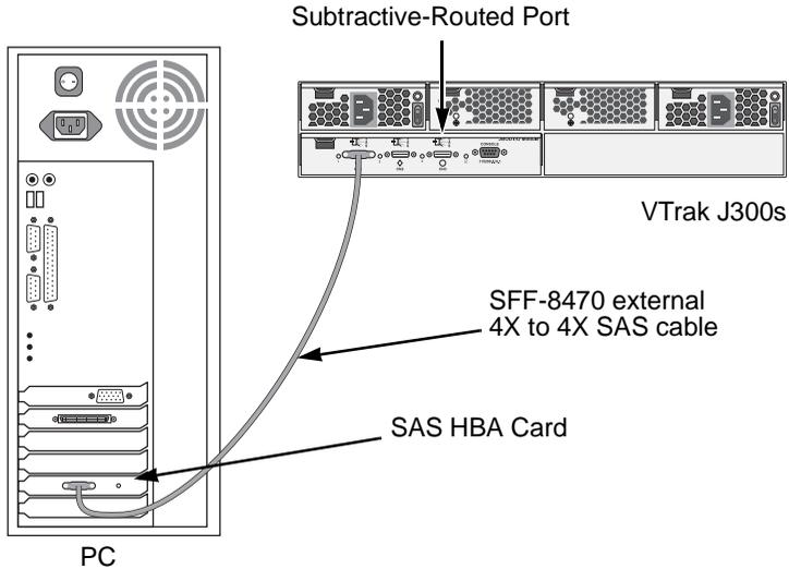
**Figure 11. An example of a basic DAS connection between one Host PC and one VTrak J300s unit**
