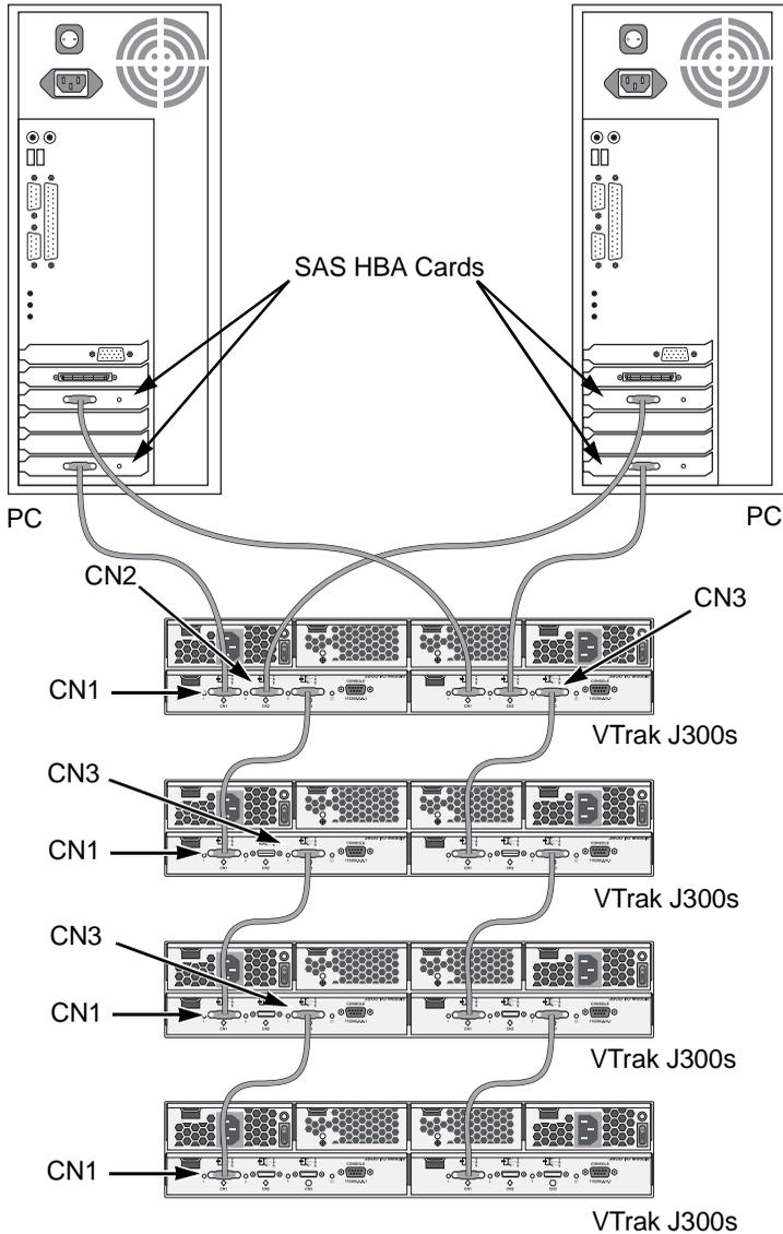
**Figure 13. An example of a redundant DAS connection between two Host PCs and four cascaded VTrak J300s units**
