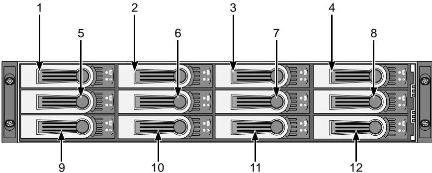
**Figure 8.** J300s unit disk drive carriers are numbered as shown
