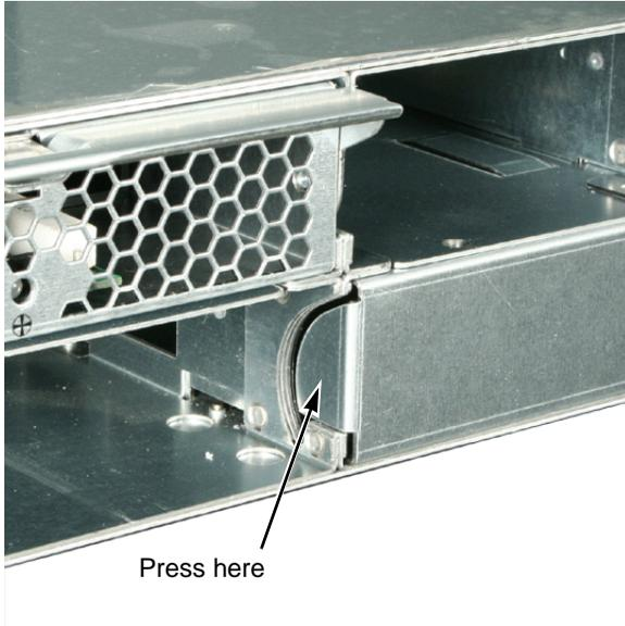
Or, remove the existing I/O module, then press on side of the blank to push it out of the slot (see above). Replace the existing I/O module. You can discard the blank and the five screws. They are not used with the second I/O module.
