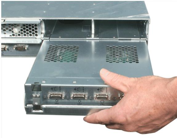
8. Install the second I/O module into the open slot (see above). Push the I/O module all the way in, then raise the handle until it locks the I/O module into place.
