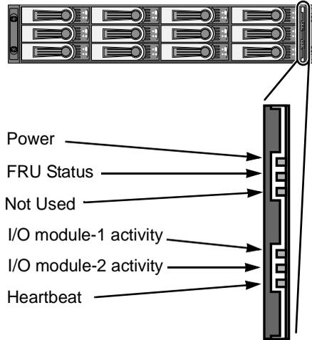
**Figure 15. VTrak J300s front panel LED display**
