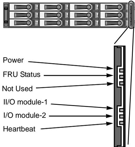
**Figure 1. VTrak J300s front panel LED display**
