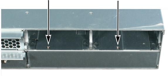
5. Remove the two screws holding the blank from the top, inside the open slots of the J300s unit (see above).
