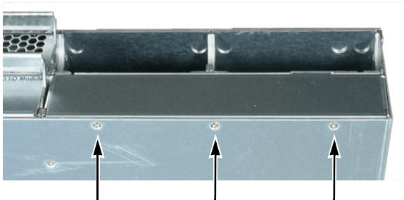
6. Remove the three screws holding the blank from the bottom of the J300s unit (see above).
