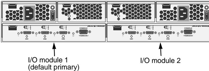
**Figure 9. VTrak J300s has one or two I/O modules**
