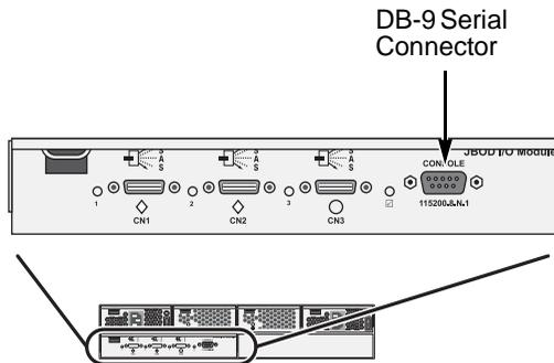
**Figure 14. A serial connector is located on the I/O module**
