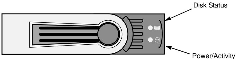
**Figure 16. VTrak J300s disk carrier LEDs**
