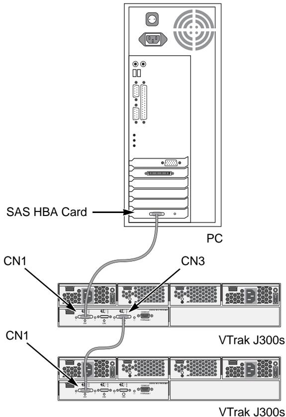
**Figure 12. An example of a cascaded DAS connection between one Host PC and three VTrak J300s units**
