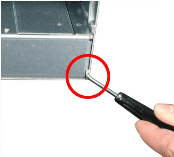
7. Insert a small screwdriver into the gap in the lower right corner of the J300s unit and gently pry the blank out of the housing (see above).
