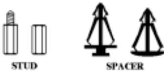
**Figure 3-3. The outline of stud and spacer**
