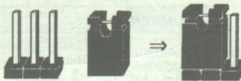
Figure 2 - 1 Jumper with Pins Shorted
