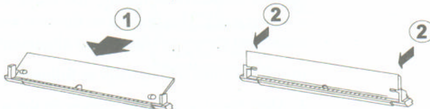
Figure 3-2. Installing a SIMM Module
