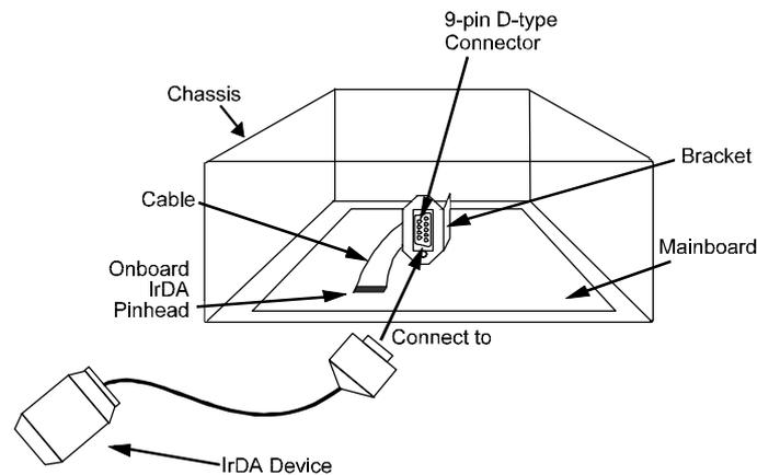
The serial port COM2 on this mainboard is designed to be a IR compliant port. If you wish to install the IR connection feature, you need to adjust the BIOS option for high-speed performance. Please read page 50 of this manual.
