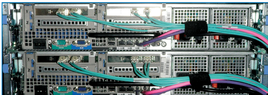
Figure 2. Simplified server connectivity using 10 Gigabit Ethernet.
