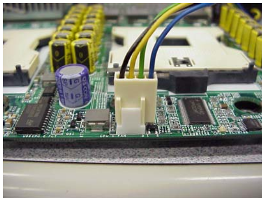
Figure 2: 4-pin fan connector plugged into the 3-pin fan header for Processor 1
