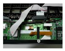
Please turn on the power. And then, please make sure the LCD backlight illuminate. If it does not illuminate, please check the connection to the LCD UNIT.
