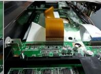
Connect the wiring to the Main Board.
