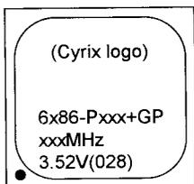
The bottom line of the mark on the processor contains a code 028 that identifies the voltage level type. If the code is 016 or others, or no marking then please contact your dealer.
