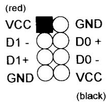
**CAUTION:** Plug wire into wrong connector will DAMAGE USB devices and mainboard.
